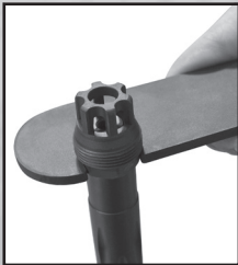
Attach sRx™ Mini Muzzle Brake to barrel using included wrench.
